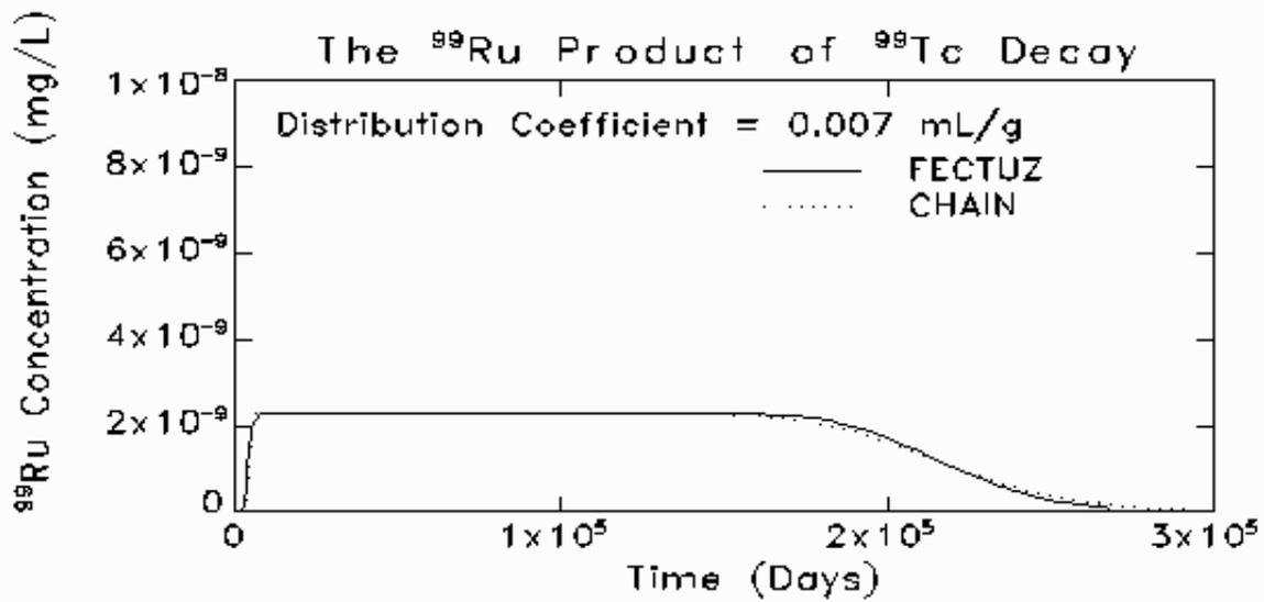
Figure 3.3. Base case simulations of the daughter product --  $^{99}\text{Ru}$  of  $^{99}\text{Tc}$  breakthrough (through the unsaturated zone) with a distribution coefficient of 0.007 mL/g using FECTUZ, and CHAIN models.
