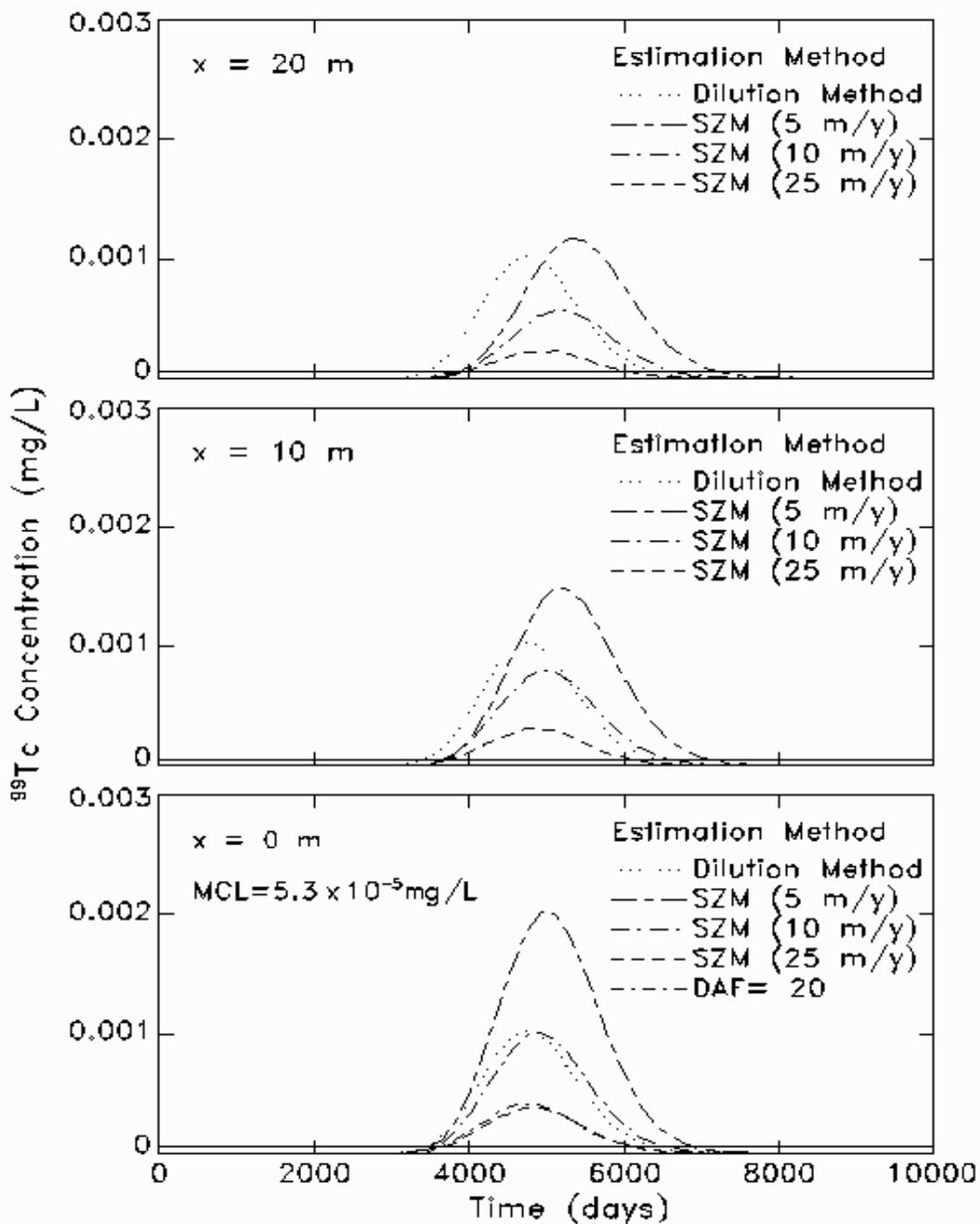
Figure 3.4. Base case prediction of <sup>99</sup>Tc concentration at the receptor well by employing dilution factor method and using saturated zone model (SZM) -- FECTUZ. The numbers in the parentheses are ground water velocity. The solid lines are used to represent the MCL ( $5.3 \times 10^{-5}$  mg/L) level.
